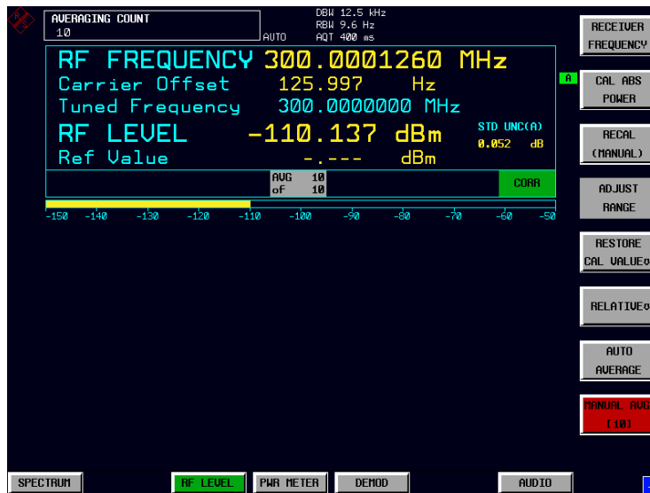
Fig.2-7 Tuned RF Level measurement at low levels
